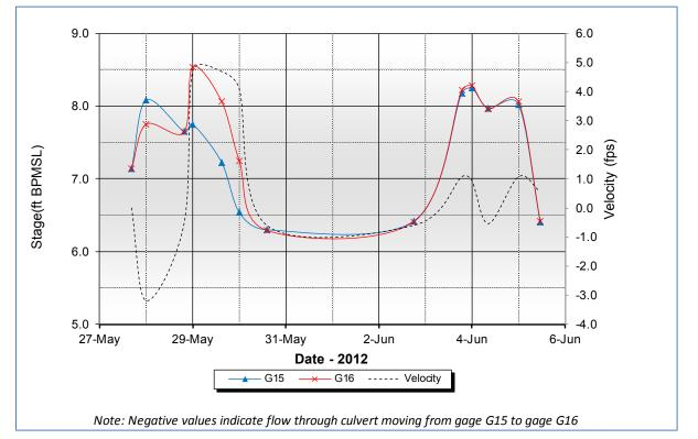
Graph 5.8: Indirect Velocity v. Observed Stage, CD4 Road Culverts near G15/G16
