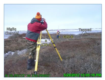
Photo 3.4: Surveying temporary indirect-read gages (G20) to BPMSL elevation; gage A is nearest to the channel centerline; May 29, 2012
