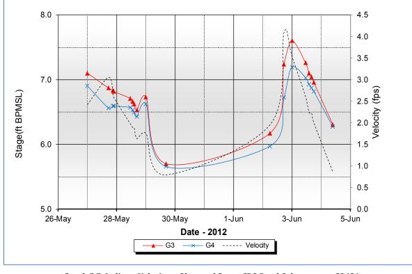
Graph 5.7: Indirect Velocity v. Observed Stage, CD2 Road Culverts near G3/G4
