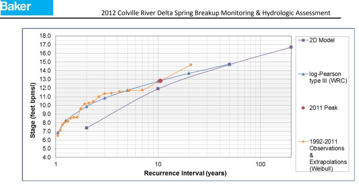
Graph 5.21: G18 Stage Frequency Analysis, 2D Model Results, and 2012 Observed Data
