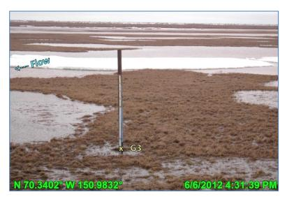
Photo 3.3: Permanent direct-read staff gage G3 near CD2 road swale bridges; June 6, 2012
