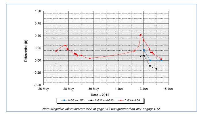
Graph 5.3: CD2 Road Water Surface Elevation Differential
