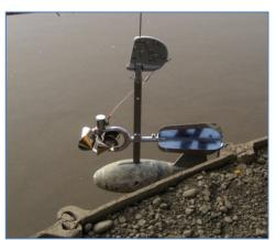
Photo 3.5: Price AA velocity meter and 30-Pound Columbus-Type sounding weight (*Baker file photo*)
