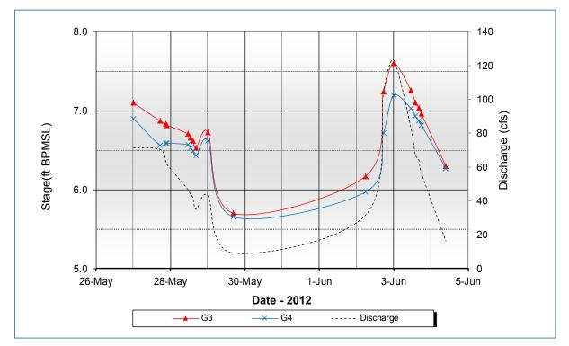
Graph 5.12: Indirect Discharge v. Observed Stage, CD2 Road Culverts near G3/G4
