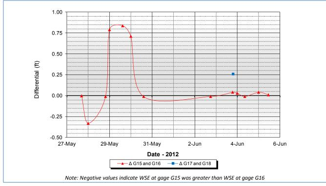
Graph 5.4: CD4 Road Water Surface Elevation Differential
