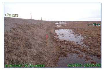
Photo 4.60: Lath defining the high water mark on the south side of CD2 road; June 6, 2012
