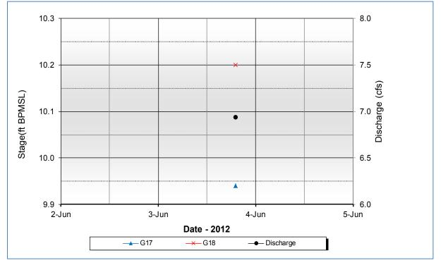
Graph 5.14: Indirect Discharge v. Observed Stage, CD4 Road Culverts near G17/G18
