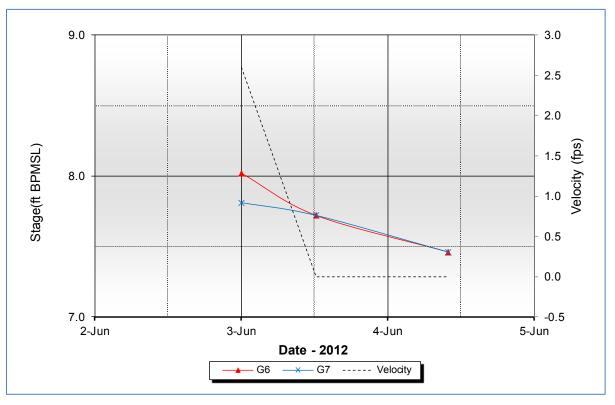
Graph 5.5: Indirect Velocity v. Observed Stage, CD2 Road Culverts near G6/G7
