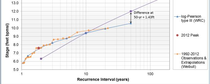
Graph 5.20: G3 Stage Frequency Analysis, 2D Model Results, and 2012 Observed Data
