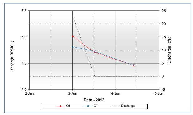
Graph 5.10: Indirect Discharge v. Observed Stage, CD2 Road Culverts near G6/G7
