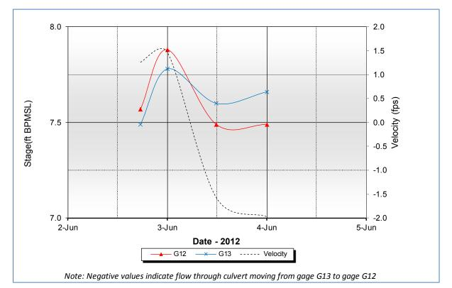
Graph 5.6: Indirect Velocity v. Observed Stage, CD2 Road Culverts near G12/G13
