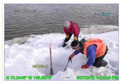
Photo 3.2: Reading water level off a staff gage at MON9; May 27, 2012
