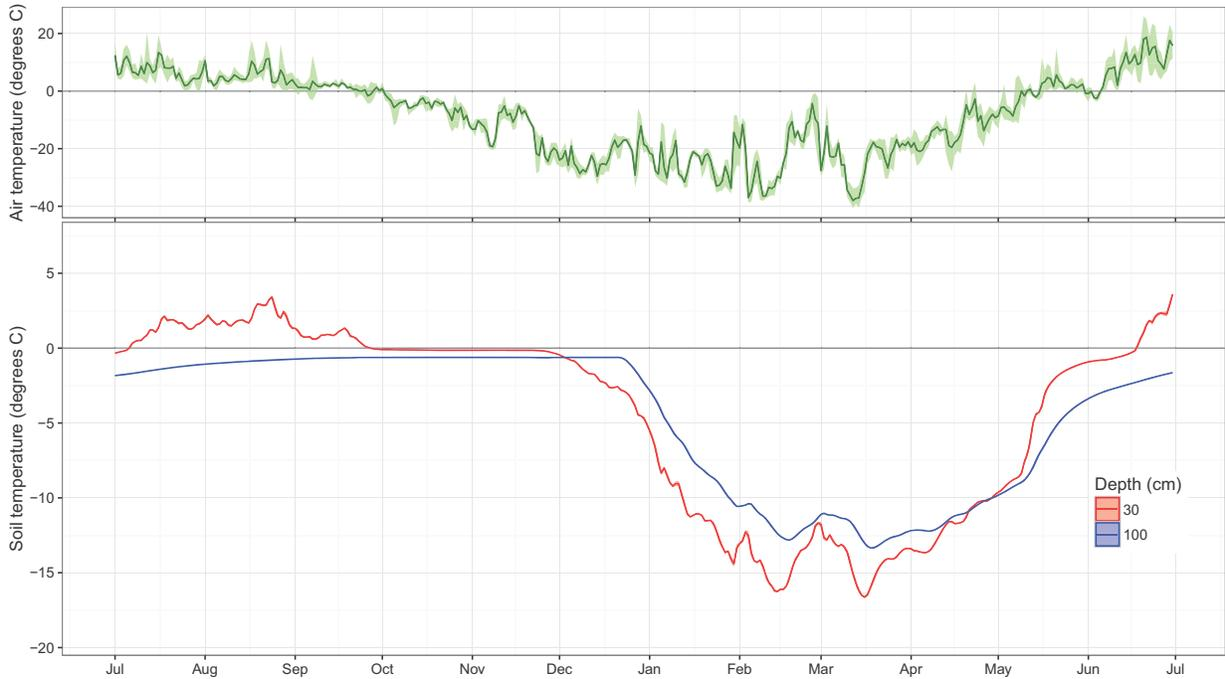
Appendix B-1. Time series of daily median soil temperature at 30 cm and 100 cm at Permafrost Monitoring Plot rn-pc01 (hobo serial number 10392122) and average daily air temperature at the Alpine weather station, CD5 Habitat Monitoring Study, northern Alaska, July 2014–June 2015.
