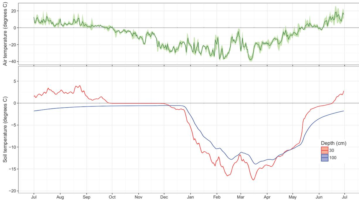
Appendix B-6. Time series of daily median soil temperature at 30 cm and 100 cm at Permafrost Monitoring Plot rs-pc11 (hobo serial number 10392132) and average daily air temperature at the Alpine weather station, CD5 Habitat Monitoring Study, northern Alaska, July 2014–June 2015.
