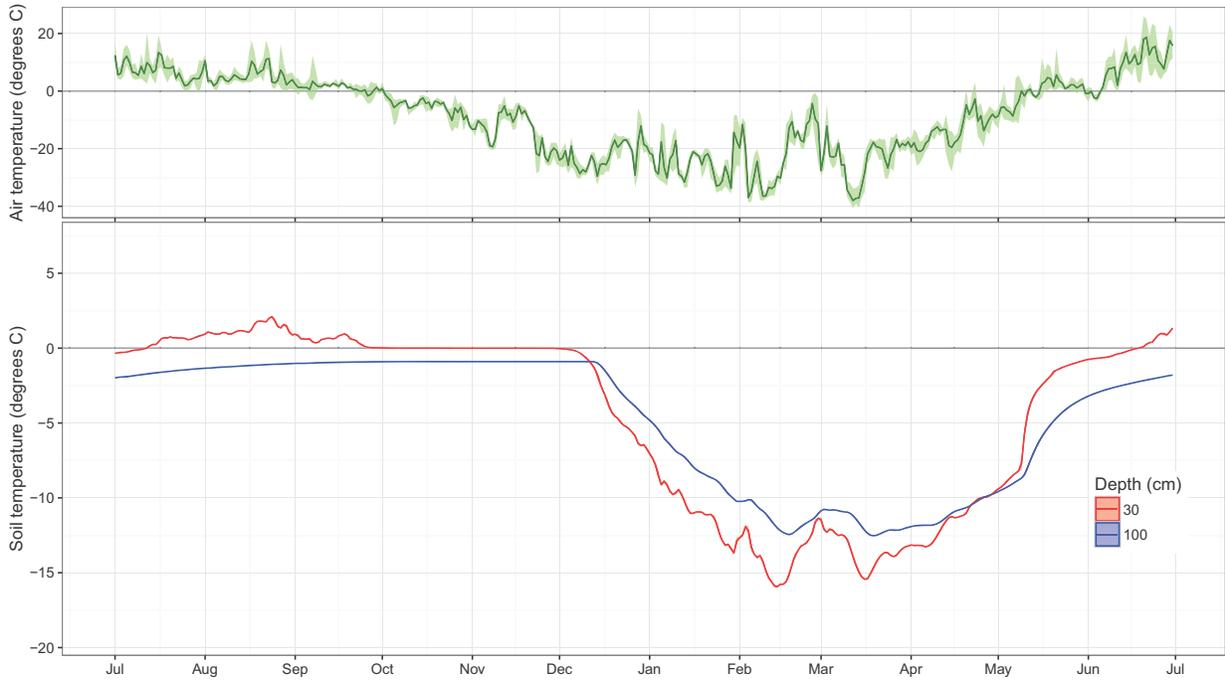
Appendix B-15. Time series of daily median soil temperature at 30 cm and 100 cm at Permafrost Monitoring Plot ts-pc13 (hobo serial number 10392134) and average daily air temperature at the Alpine weather station, CD5 Habitat Monitoring Study, northern Alaska, July 2014–June 2015.
