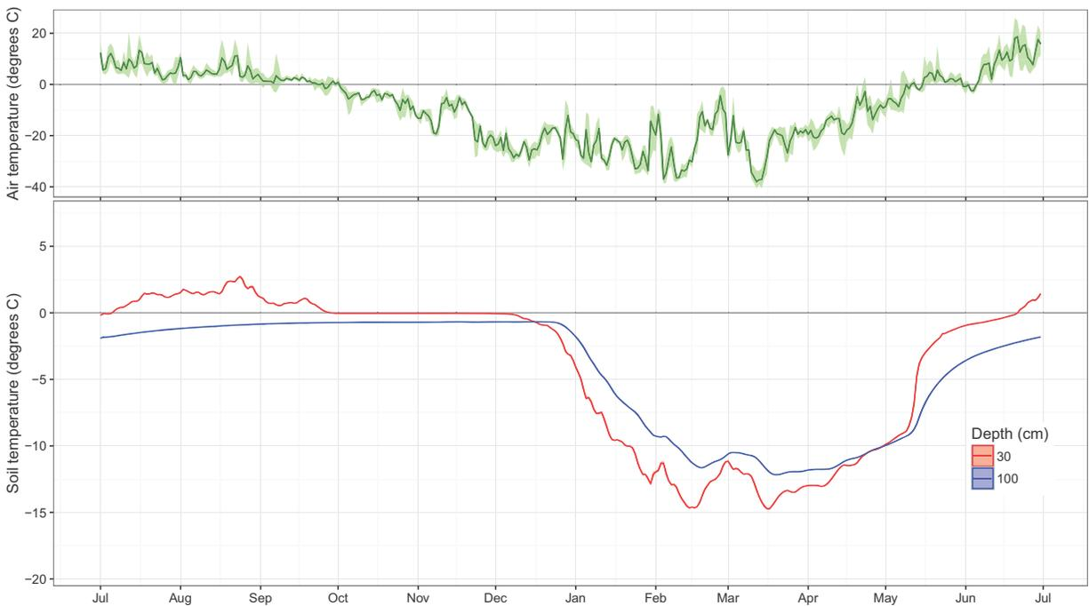
Appendix B-8. Time series of daily median soil temperature at 30 cm and 100 cm at Permafrost Monitoring Plot tn-pc04 (hobo serial number 10392125) and average daily air temperature at the Alpine weather station, CD5 Habitat Monitoring Study, northern Alaska, July 2014–June 2015.
