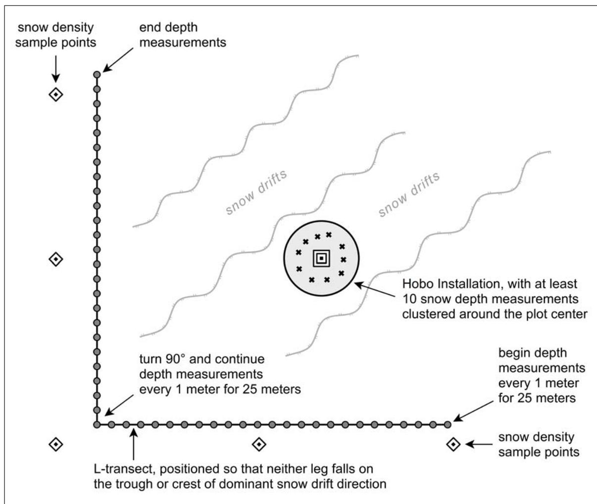
Figure 5. Schematic of snow survey plot design, CD5 Habitat Monitoring Study, northern Alaska, 2015.
