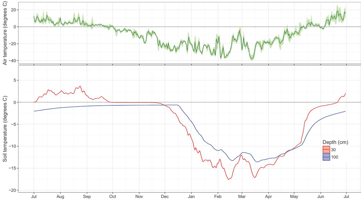
Appendix B-9. Time series of daily median soil temperature at 30 cm and 100 cm at Permafrost Monitoring Plot tn-pc05 (hobo serial number 10392126) and average daily air temperature at the Alpine weather station, CD5 Habitat Monitoring Study, northern Alaska, July 2014–June 2015.
