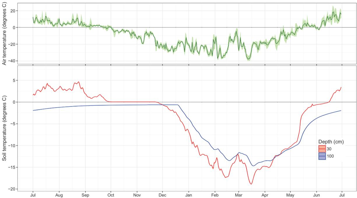
Appendix B-4. Time series of daily median soil temperature at 30 cm and 100 cm at Permafrost Monitoring Plot rs-pc09 (hobo serial number 10392130) and average daily air temperature at the Alpine weather station, CD5 Habitat Monitoring Study, northern Alaska, July 2014–June 2015.
