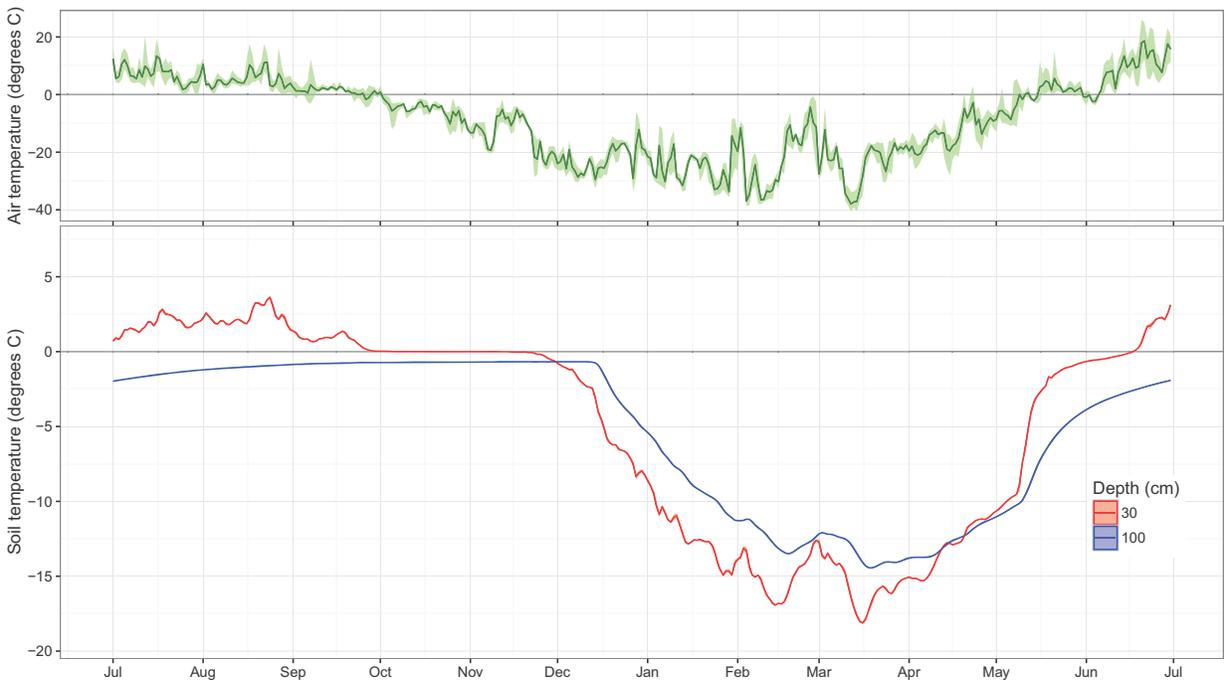
Appendix B-16. Time series of daily median soil temperature at 30 cm and 100 cm at Permafrost Monitoring Plot ts-pc14 (hobo serial number 10392135) and average daily air temperature at the Alpine weather station, CD5 Habitat Monitoring Study, northern Alaska, July 2014–June 2015.
