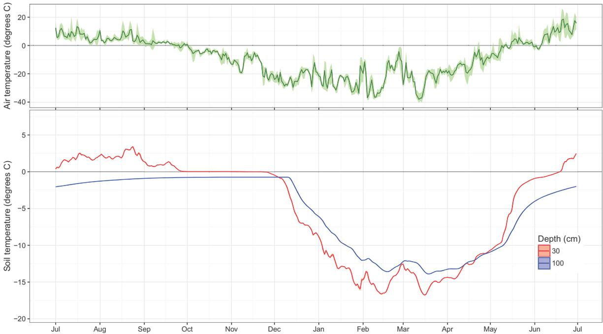
Appendix B-2. Time series of daily median soil temperature at 30 cm and 100 cm at Permafrost Monitoring Plot rn-pc02 (hobo serial number 10392123) and average daily air temperature at the Alpine weather station, CD5 Habitat Monitoring Study, northern Alaska, July 2014–June 2015.
