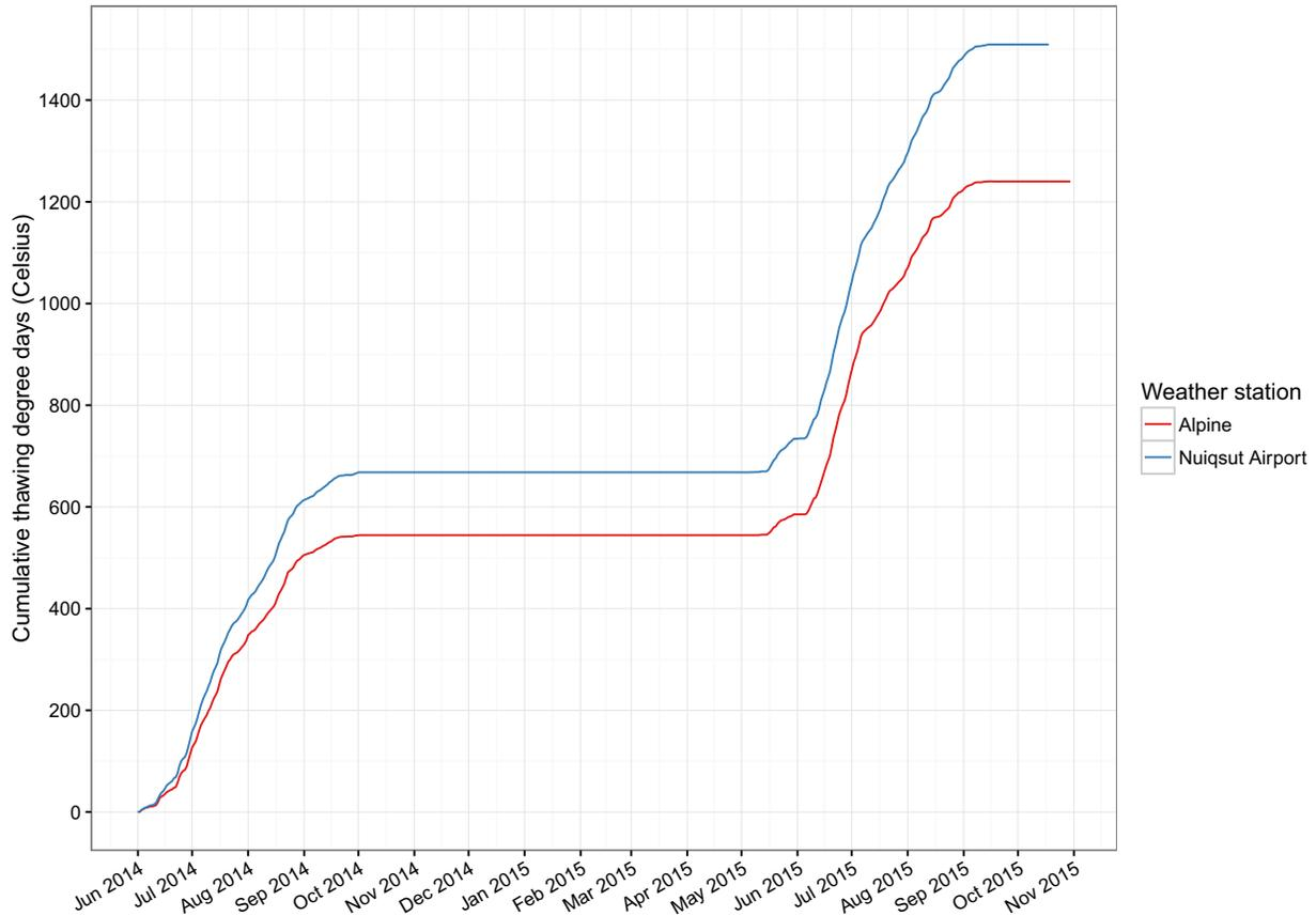
Figure 9. Cumulative thawing degree days (TDD) for the Alpine Weather Station and the Nuiqsut Airport National Weather Service Station, June 2014–September 2015.
