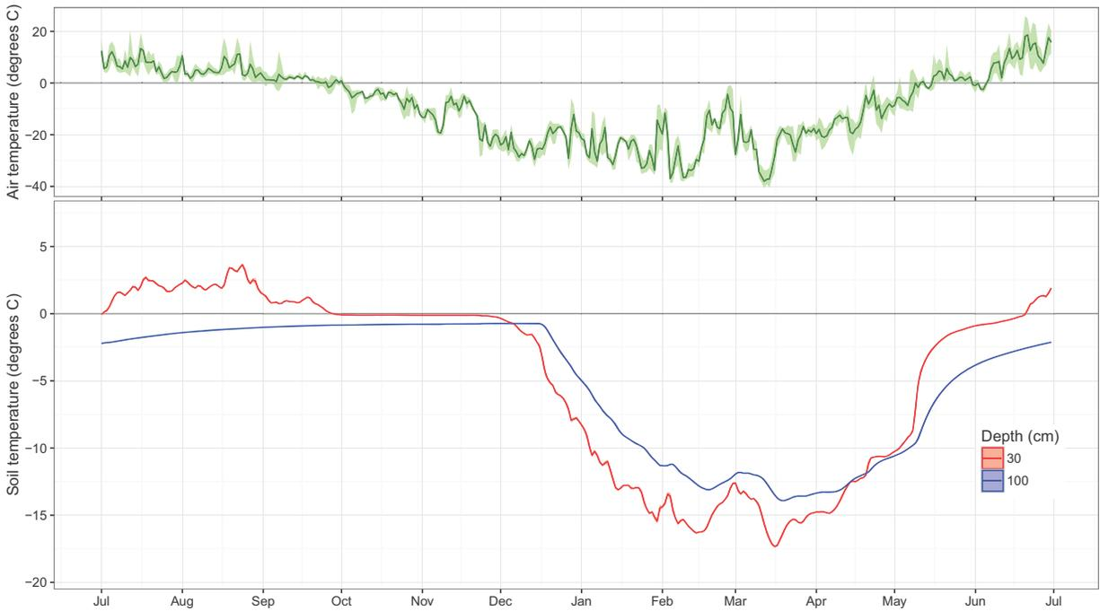
Appendix B-12. Time series of daily median soil temperature at 30 cm and 100 cm at Permafrost Monitoring Plot ts-pc07 (hobo serial number 10392128) and average daily air temperature at the Alpine weather station, CD5 Habitat Monitoring Study, northern Alaska, July 2014–June 2015.
