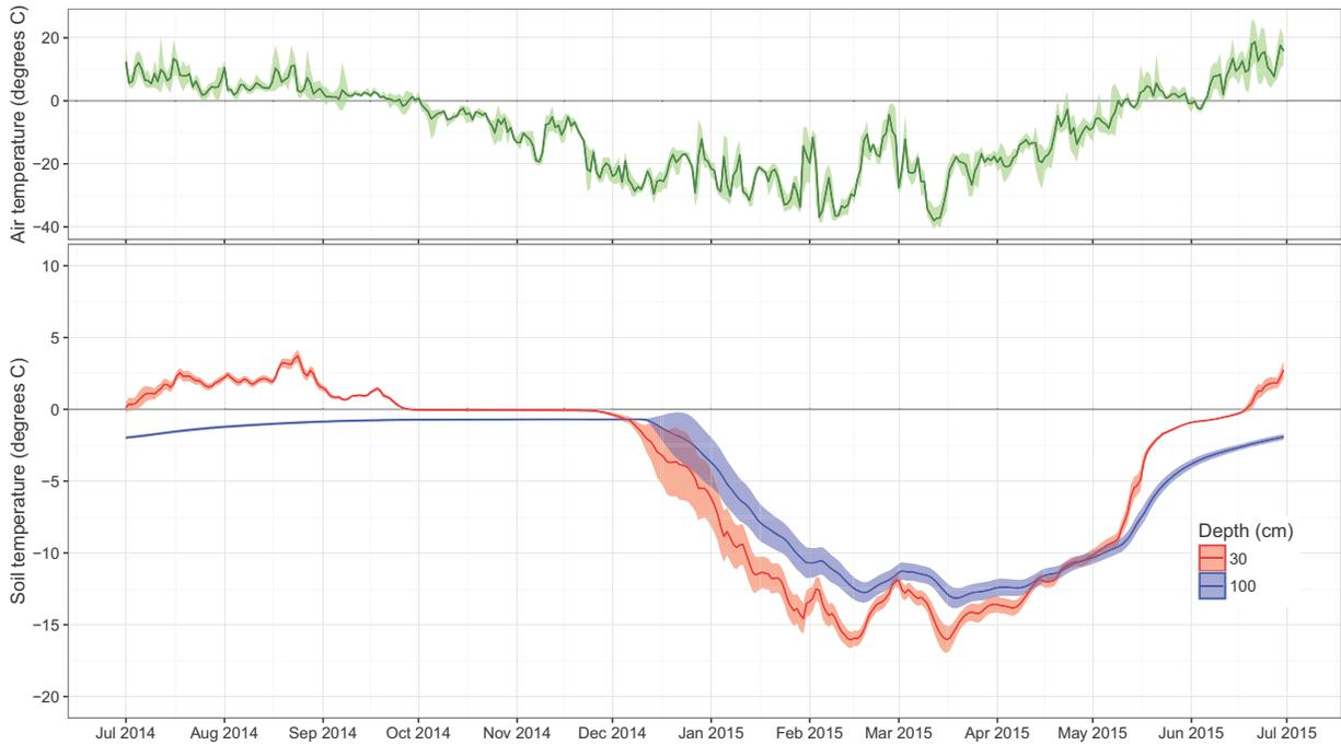
Figure 17. Time series of daily mean soil temperature and standard deviation at 30 cm and 100 cm for Reference Area North, and average daily minimum, mean and maximum air temperature, CD5 Habitat Monitoring Study, northern Alaska, July 2014–June 2015.
