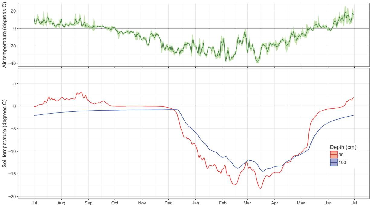
Appendix B-10. Time series of daily median soil temperature at 30 cm and 100 cm at Permafrost Monitoring Plot tn-pc06 (hobo serial number 10392127) and average daily air temperature at the Alpine weather station, CD5 Habitat Monitoring Study, northern Alaska, July 2014–June 2015.
