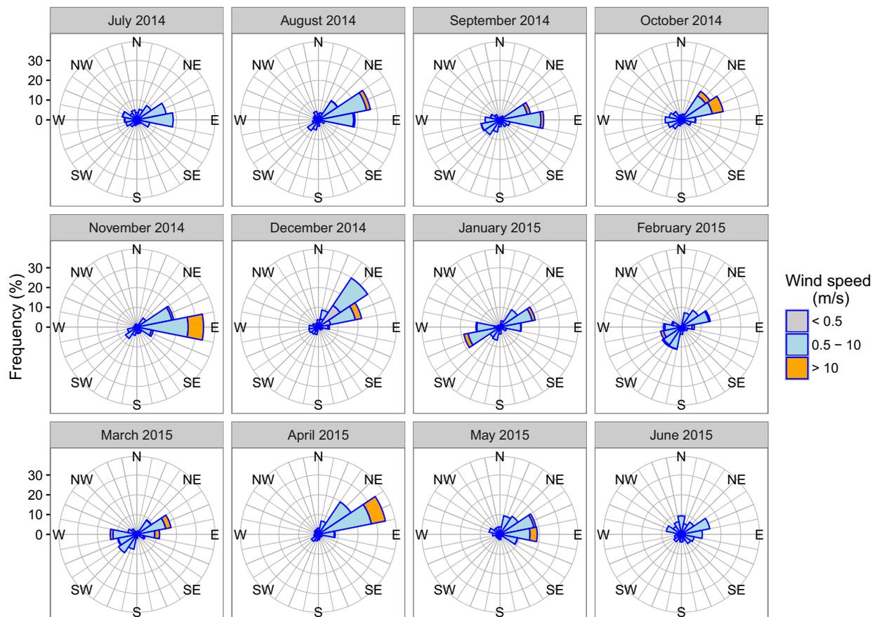
Figure 11. Charts summarizing monthly wind speed and direction at the Alpine Weather Station, Colville River Delta, northern Alaska, July 2014–June 2015.
