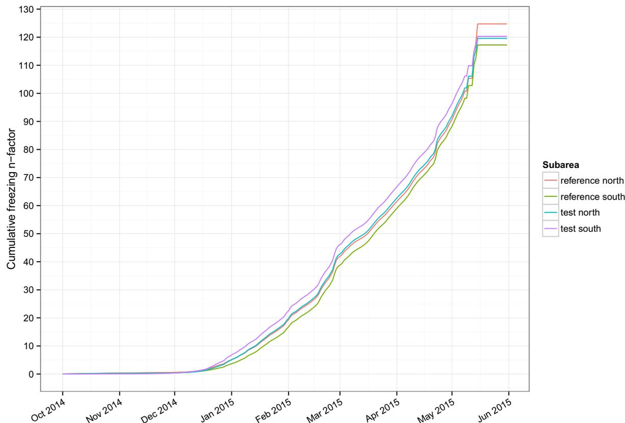
Figure 22. Average cumulative freezing n-factor at 30 cm for Permafrost Monitoring Plots in Reference Area North, Reference Area South, Test Area North, and Test Area South, CD5 Habitat Monitoring Study, northern Alaska, October 2014–May 2015. Freezing n-factors displayed in this graph are calculated as the ratio of the freezing degree days in the soil to the freezing degree days of the air using the average of the Nuiqsut Airport and Alpine Weather Station average daily air temperature.
