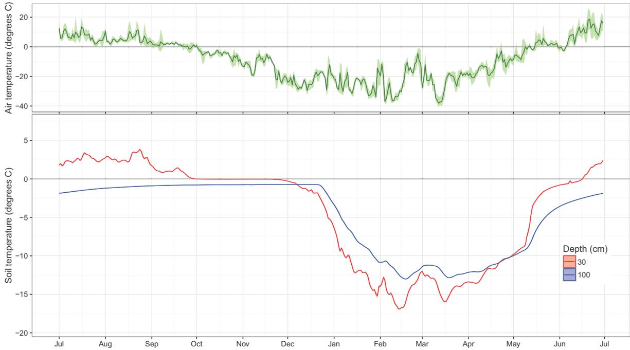
Appendix B-7. Time series of daily median soil temperature at 30 cm and 100 cm at Permafrost Monitoring Plot tn-pc03 (hobo serial number 10392124) and average daily air temperature at the Alpine weather station, CD5 Habitat Monitoring Study, northern Alaska, July 2014–June 2015.
