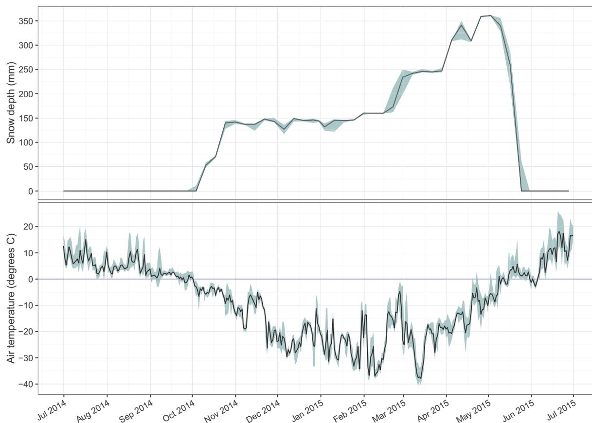
Figure 8. Median, 25th- and 75th-quartile of weekly snow depth, and average daily minimum, mean and maximum air temperature, at the Alpine Weather Station, Colville River Delta, northern Alaska, July 2014–June 2015.
