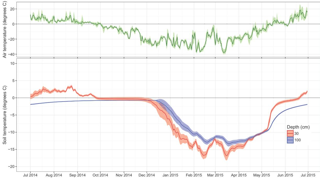
Figure 19. Time series of daily mean soil temperature and standard deviation at 30 cm and 100 cm for Test Area North, and average daily minimum, mean and maximum air temperature, and median weekly snow depth at the Alpine weather station, CD5 Habitat Monitoring Study, northern Alaska, July 2014–June 2015.
