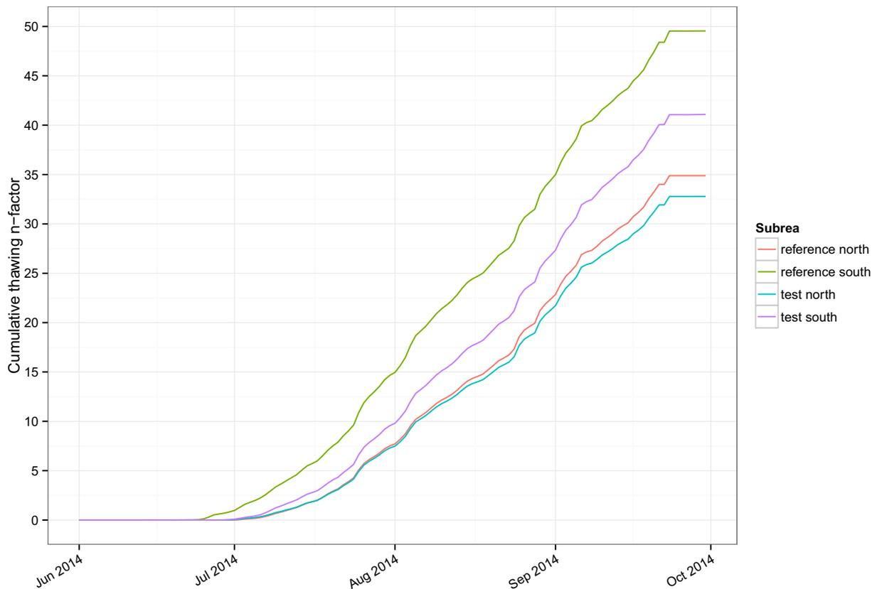
Figure 21. Average daily cumulative thawing n-factor at 30 cm for Permafrost Monitoring Plots in Reference Area North, Reference Area South, Test Area North, and Test Area South, CD5 Habitat Monitoring Study, northern Alaska, June 2014–September 2014. Thawing n-factors displayed in this graph are calculated as the ratio of the thawing degree days in the soil to the thawing degree days of the air using the average of the Nuiqsut Airport and Alpine Weather Station average daily air temperature.
