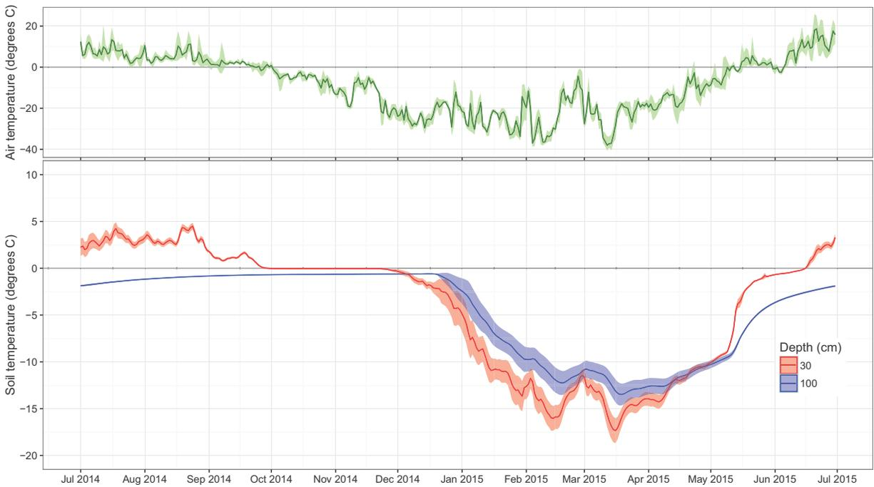
Figure 18. Time series of daily mean soil temperature and standard deviation at 30 cm and 100 cm for Reference Area South, and average daily minimum, mean and maximum air temperature, CD5 Habitat Monitoring Study, northern Alaska, July 2014–June 2015.
