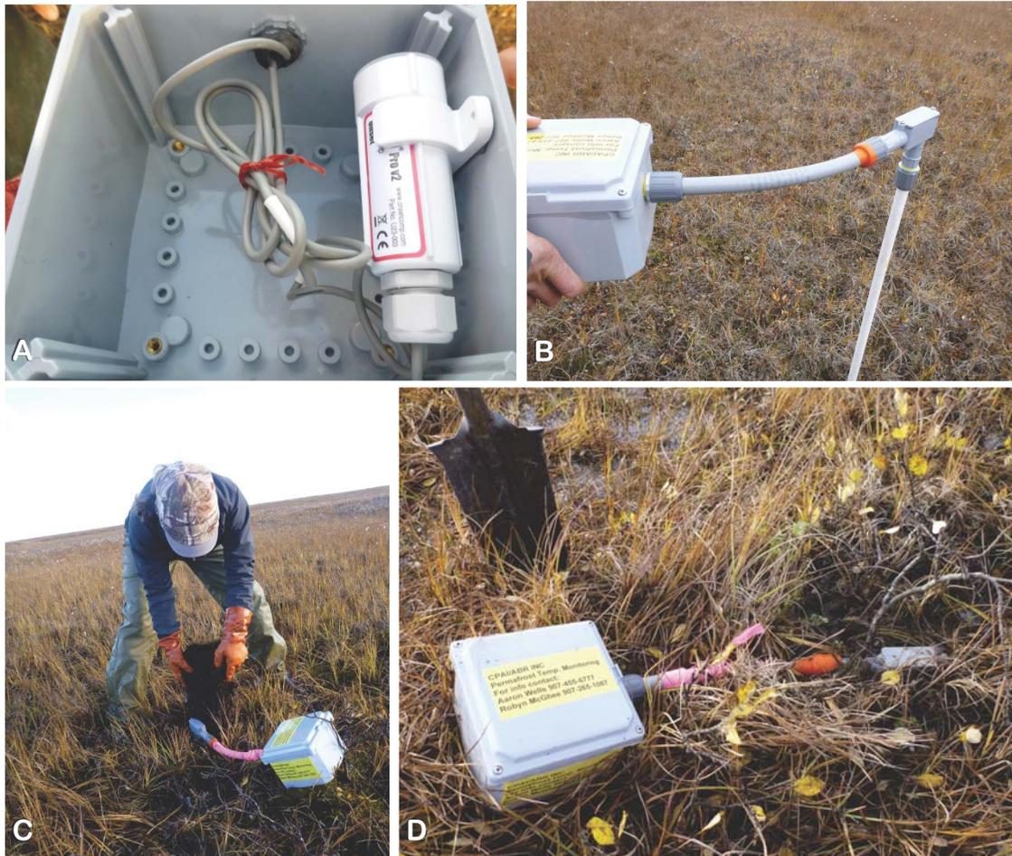
Figure 7. Temperature Logger installation and field deployment, CD5 Habitat Monitoring Study, northern Alaska, 2013–2015. Installation includes a) feeding the HOBO logger cables through the water proof box and into the PVC tube to a depth of 11.8 in (30 cm) and 39.4 in (100 cm) from the soil surface; b) sealing the box and PVC tube and reinforcing connections with waterproof tape; c) removing and restoring the surface organic mat; and d) an image of the final logger installation.
