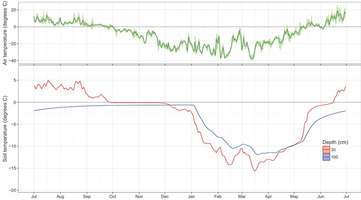
Appendix B-5. Time series of daily median soil temperature at 30 cm and 100 cm at Permafrost Monitoring Plot rs-pc10 (hobo serial number 10392131) and average daily air temperature at the Alpine weather station, CD5 Habitat Monitoring Study, northern Alaska, July 2014–June 2015.
