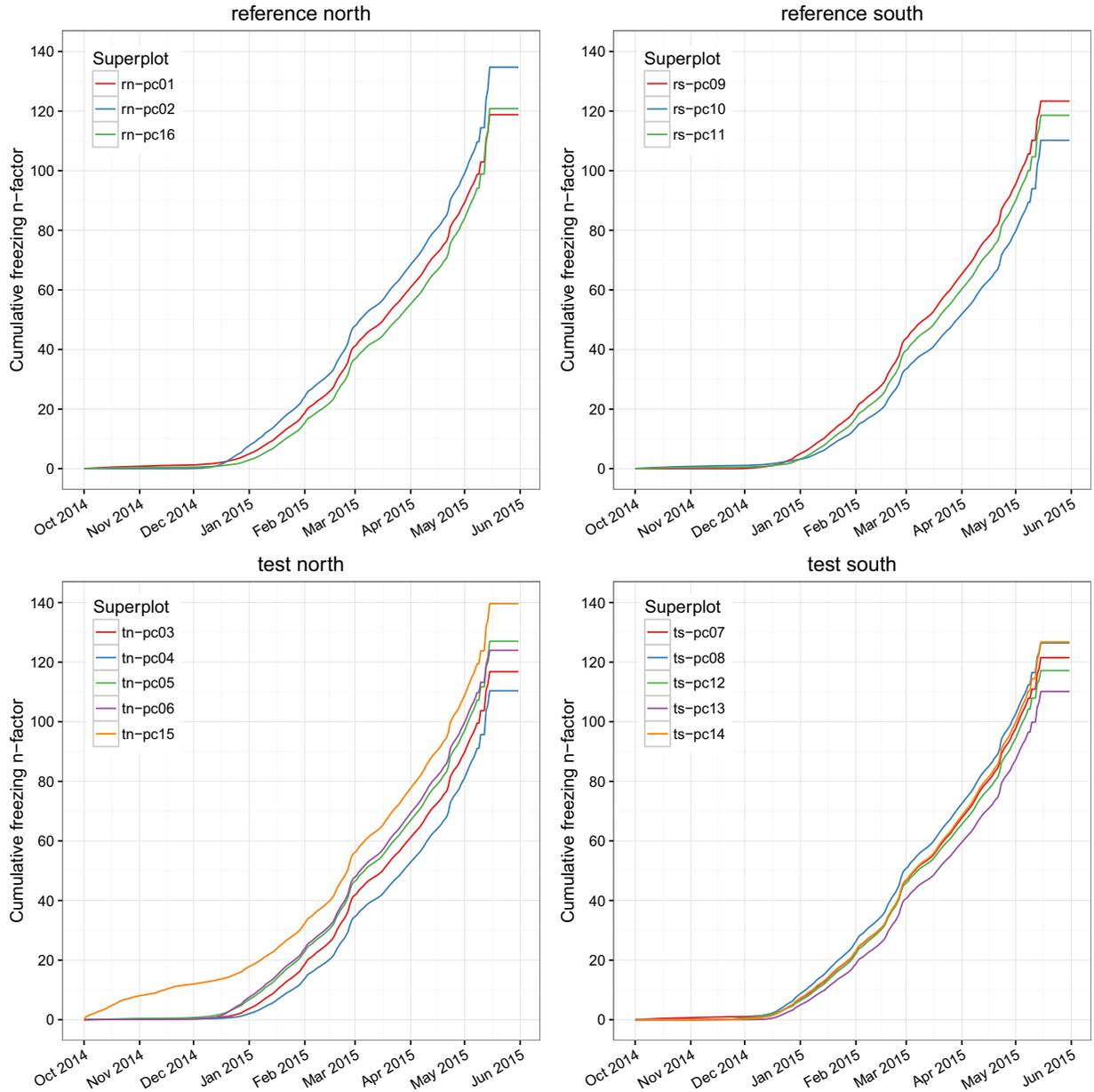
Figure 16. Daily cumulative freezing n-factor at 30 cm for each of 16 Permafrost Monitoring Plots by area, CD5 Habitat Monitoring Study, northern Alaska, October 2014–May 2015. Freezing n-factors displayed in this graph are calculated as the ratio of the freezing degree days in the soil to the freezing degree days of the air using the average of the Nuiqsut Airport and Alpine Weather Station average daily air temperature.
