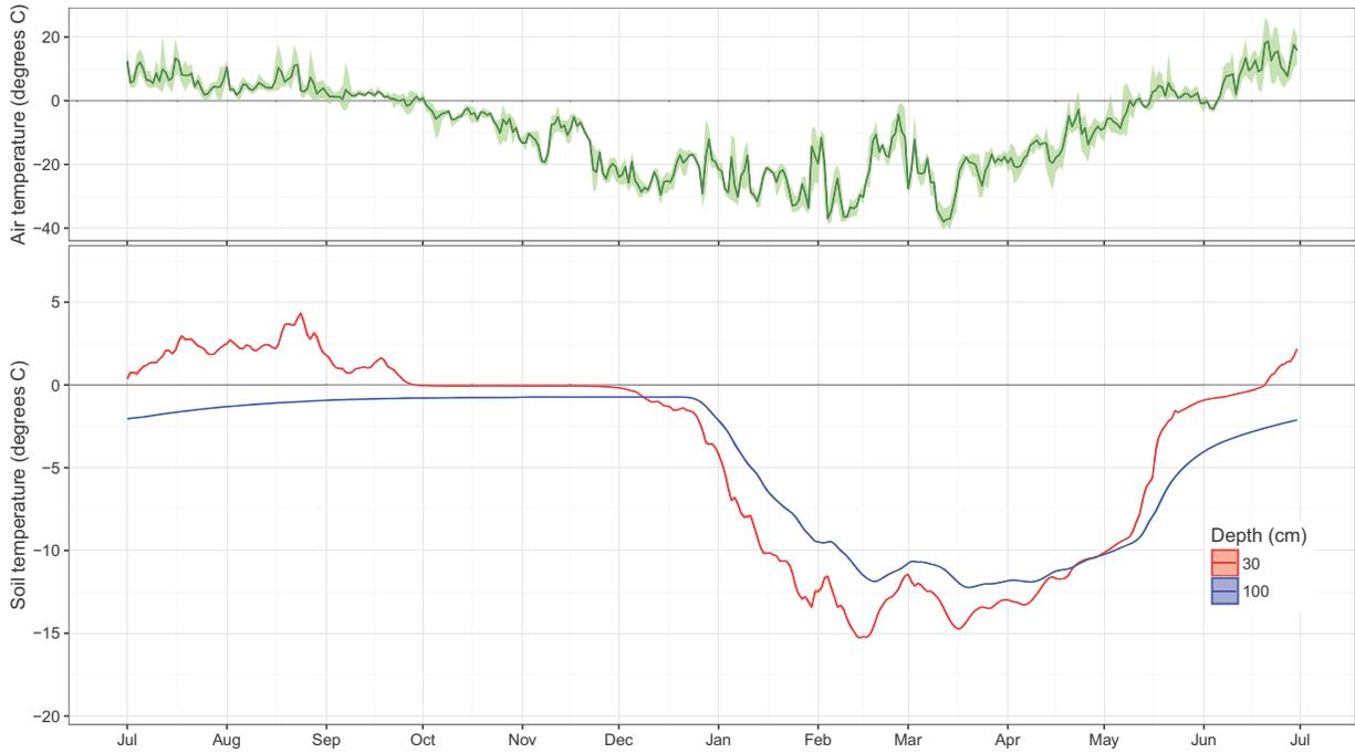
Appendix B-3. Time series of daily median soil temperature at 30 cm and 100 cm at Permafrost Monitoring Plot rn-pc16 (hobo serial number 10392137) and average daily air temperature at the Alpine weather station, CD5 Habitat Monitoring Study, northern Alaska, July 2014–June 2015.
