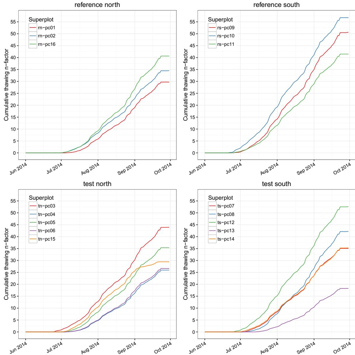
Figure 15. Daily cumulative thawing n-factor at 30 cm for each of 16 Permafrost Monitoring Plots by area, CD5 Habitat Monitoring Study, northern Alaska, June 2014–September 2014. Thawing n-factors displayed in this graph are calculated as the ratio of the thawing degree days in the soil to the thawing degree days of the air using the average of the Nuiqsut Airport and Alpine Weather Station average daily air temperature.
