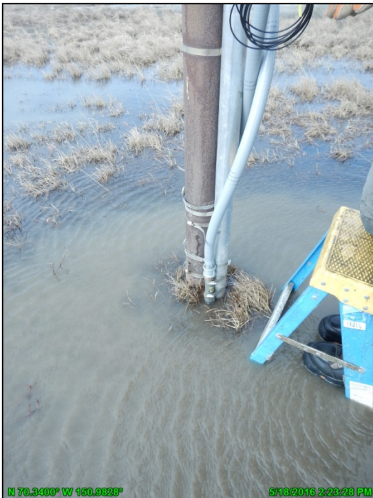
Photo 2.8: Pressure transducer connected to datalogger at gage G3; May 18, 2016
