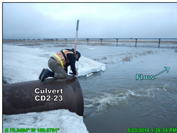
Photo 4.9: Culvert CD2-23 direct discharge measurement, looking northwest; May 23, 2016
