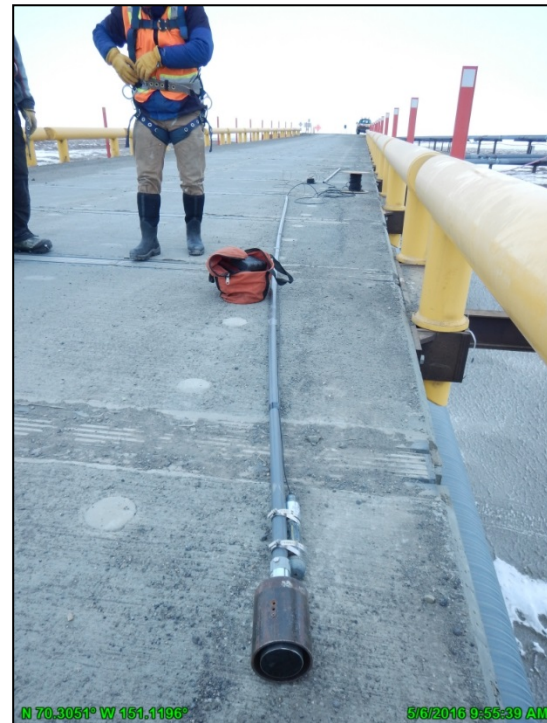
Photo 2.9: Single beam sonar and pressure transducer at Nigliagvik Bridge; May 6, 2016
