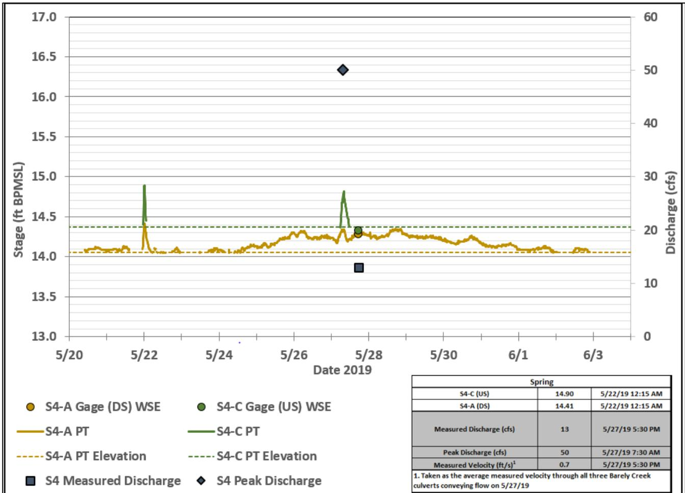
Graph 4.9: Barely Creek Culvert Battery Spring Breakup Stage, Velocity, & Discharge
