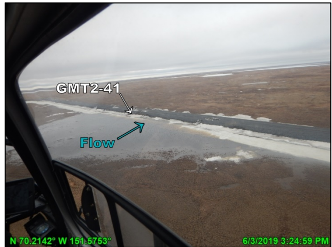
Photo F.13: Differential ponding near culvert GMT2-41, looking west; June 3, 2019
