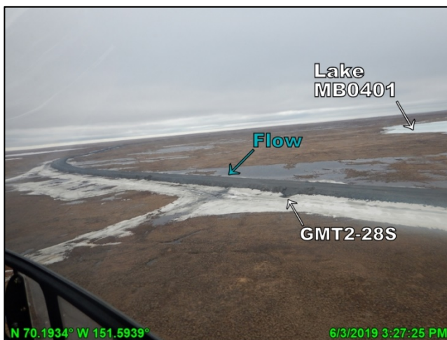
Photo 3.5: Ponded water on the north side of GMT2/MT7 access road near culvert GMT2-28, looking west; June 3, 2019
