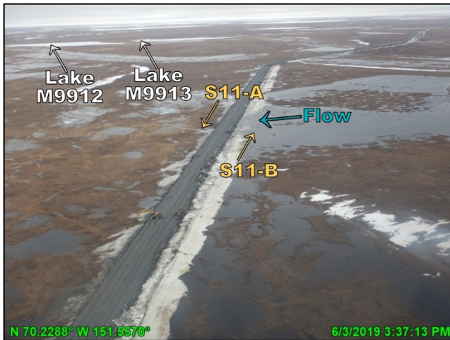
Photo F.12: Differential ponding near S11, looking north; June 3, 2019
