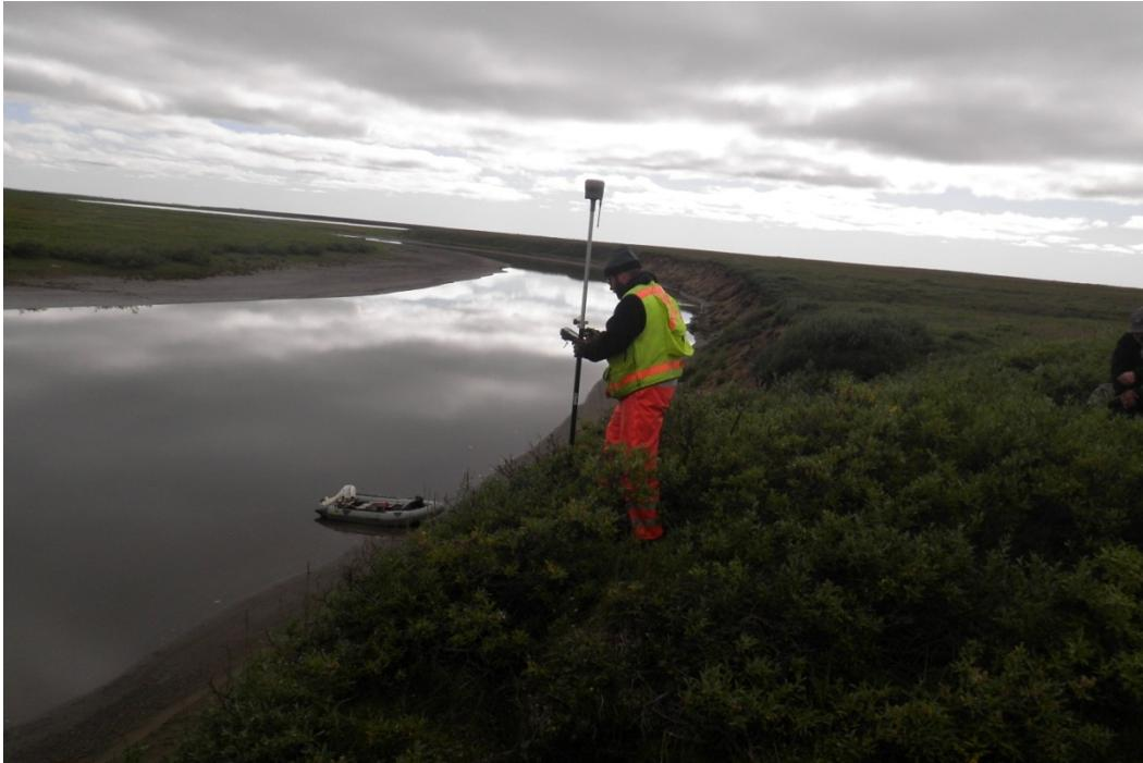
**Photo 2: Surveying the edge of the west bank of the Nigliagvik with Real Time Kinematic GPS; August 21, 2013**
