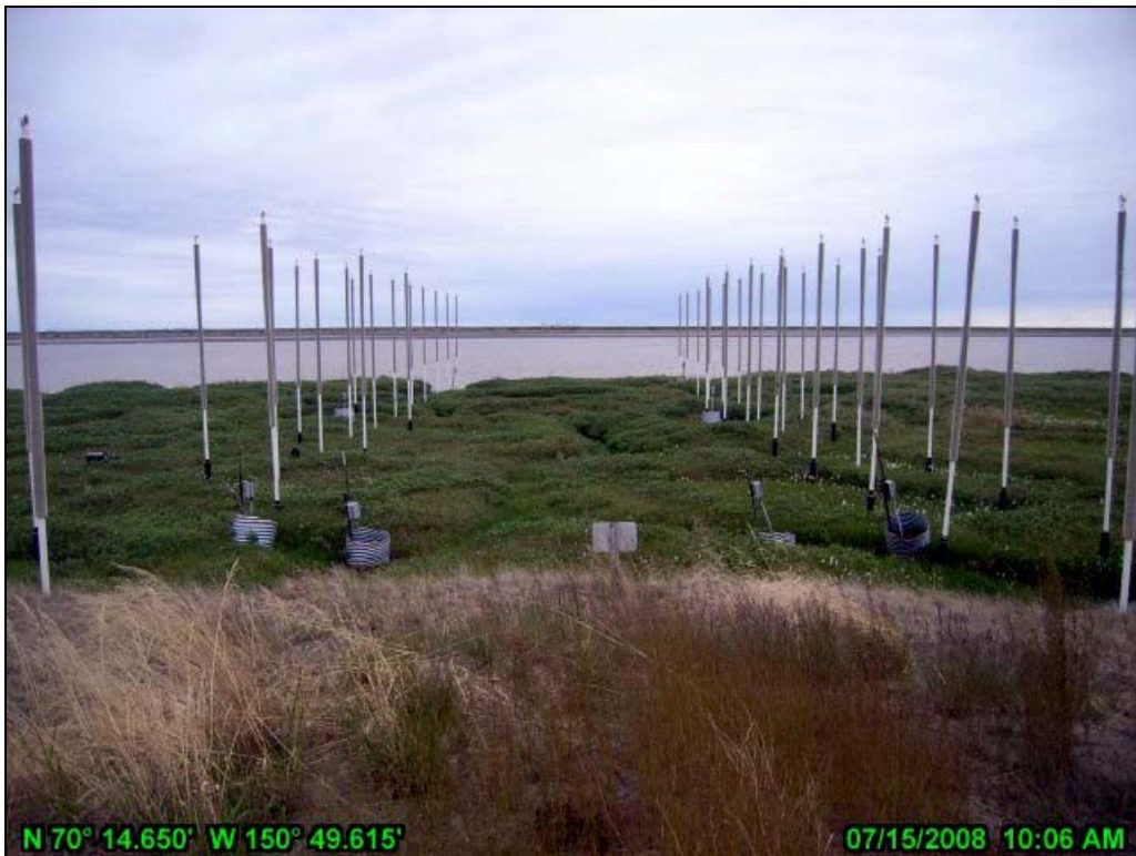
Photo A-9 HDD East, July 15, 2008. Thermosyphons and polygon trough at HDD East, looking west.
